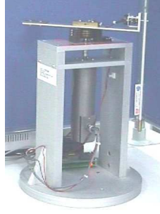
Figure 1: A version of the Furuta pendulum, available from KentRidge Instruments ( http://www.kri.com.sg ) as product PP300
