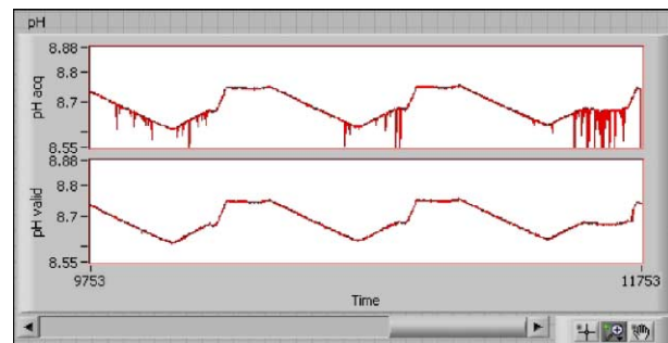
Figure 5 | A sample of pH data before (above) and after (below) the PDV processing. The many artefacts, appearing as large spikes in the original signal, have been entirely eliminated in the validated data.
