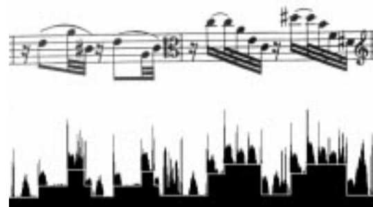
Figure 3. Level 1: the gray line reports different offset levels corresponding to the presence of beams.
