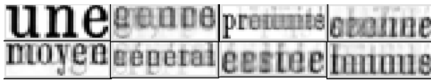
Fig. 1. Eight prototypes obtained from a SOM map trained with the standard training algorithm. Apart from very common words (e.g. "une") the prototypes do not correspond to actual words.
